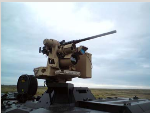
Integration of ROWS – Remote Overhead Weapon Station – Protector med HMG cal .50 (20 mm AKA to be phased out)
